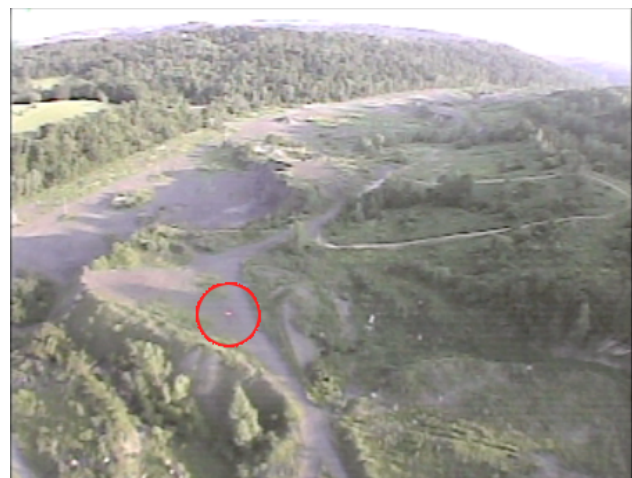
Figure 2. A UAV video sample containing the one meter square orange targets used in the experiment (circled in red). The target can be distinguished from the natural surroundings by its unique color.
