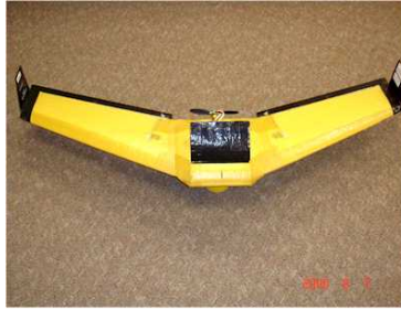
Figure 14: Procerus UAV with 60" wingspan used for live flight experiments.
