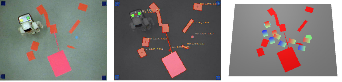
Fig. 4. Top-down view of the walking environment (left), vision system output (center), and corresponding environment map with current footstep plan generated (right).
