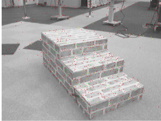
Figure 6.17: SIFT keypoints extracted from camera image while attempting to establish the pose of the stairs in the view. Found keypoints ( red ). Subset of found keypoints matched by Best-Bin-First search ( yellow ) to keypoints from a model image, Subset of matched keypoints determined to be inliers by RANSAC ( green ). Around 40 keypoints are ultimately kept.
