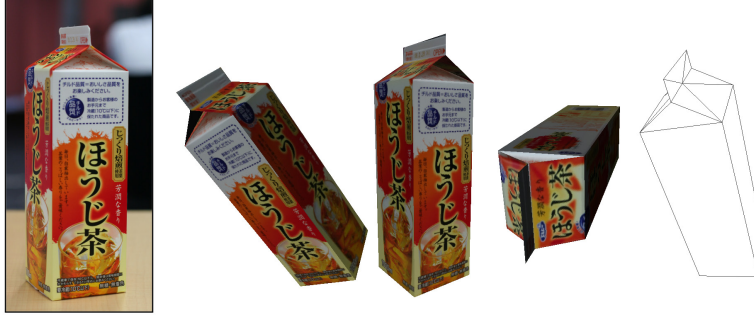
Figure 6.5: Image-based modeling of objects of interest. One of four input images used for modeling the tea carton ( left ). Three sample views of the resulting 3D model ( center ). Hidden-line wireframe version of the model used for tracking ( right ).
