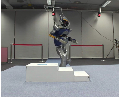
Figure 8.1: HRP-2 executing a stairclimbing motion planned in a perception-agnostic manner. The stairs move outside the robot’s view during locomotion and tracking subsequently fails.
