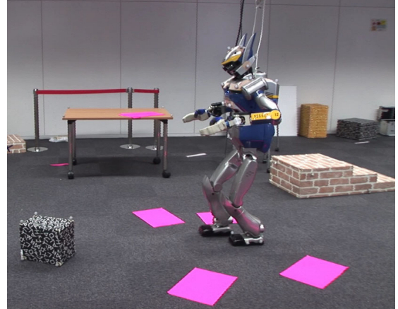
Fig. 1. The HRP-2 humanoid navigating autonomously through a set of obstacles during vision-guided walking.
