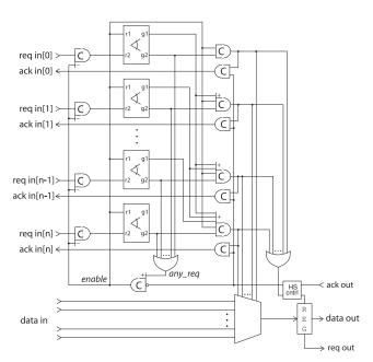
Figure 3: Handshake-multiplexer implements an access tree node.
