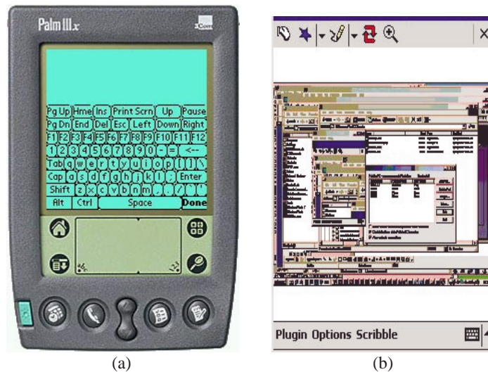
Fig. 1. Palm (a) and PocketPC (b) Remote Commander screens. The PocketPC version displays a PC's screen image.
