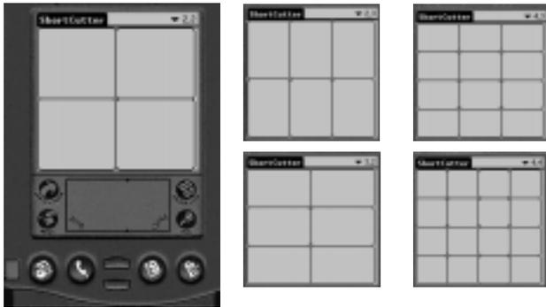
**Figure 1.** Left: a picture of a Palm Pilot (the WorkPad is similar) showing the 2x2 layout of buttons. Right: the screens for 3x2, 2x3, 4x3 and 4x4. The other layouts are similar.
