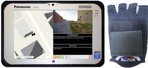
Fig. 3. An illustration of the Multi-Modal Interface (MMI) for human-robot interaction. The MMI accepts input in the form of speech and/or gesture and visualizes the state of the intelligence architecture. The MMI Visual Display illustrates a “screen the back of the building” command. The robot status shown in the COMMANDS and STATUS sections indicate the command is still running and the robot is currently searching.
