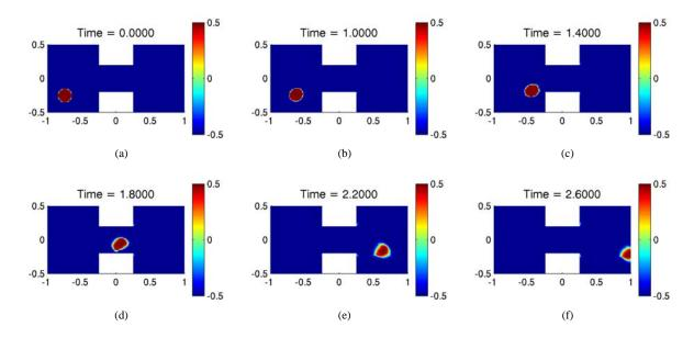
FIG. 6.3. The evolution of the phase function for a cell flowing through a notched channel. In this example, there is an elastic membrane present at the interface.
