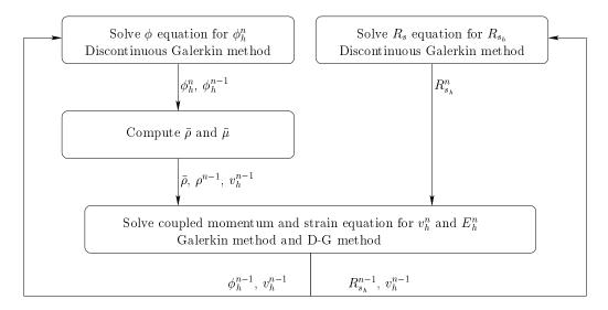
FIG. 4.1. The solution methodology for modeling the motion of two fluids separated by an elastic membrane. Lagging the velocity in the convective terms of all four systems of equations decouples the phase equation and the rotation from the momentum and strain equations.
