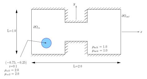
FIG. 6.1. The schematic of the geometry and material properties for the simulation of a cell, both with and without an elastic membrane, flowing through a notched channel.
