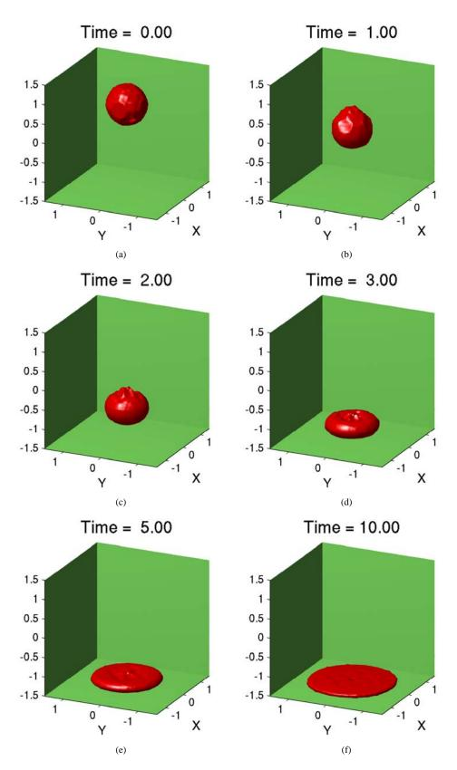
FIG. 7.1. The isosurface,  $\phi = 0$ , of the phase variable for a three-dimensional falling drop simulation without an elastic membrane.
