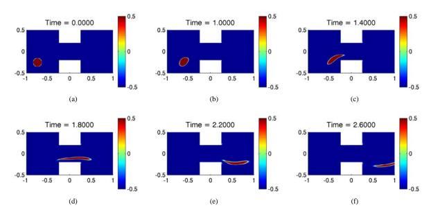
FIG. 6.2. The evolution of the phase function for a cell flowing through a notched channel at times (a) t = 0.0, (b) t = 1.0, (c) t = 1.4, (d) t = 1.8, (e) t = 2.2 and (f) t = 2.6. In this example, there is no elastic membrane present at the interface.
