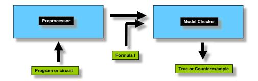
Figure 5: A Model Checker that supports Counterexamples
