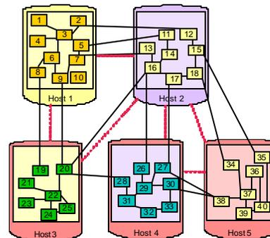
Figure 1. Example deployment architecture. A software system comprising 40 components is deployed onto five hosts. The dotted lines represent host interconnectivity; the filled lines represent software component interaction paths.
