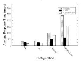
**Figure 6.** Summary of cache performance using the TPC-W benchmark. The four cases are: (i) Base TPC-W with a 10K item database, (ii) Base TPC-W with a 100K item database, (iii) Modified TPC-W with a 100K item database, (iv) Modified TPC-W with a 100K item database and a loaded back-end.
