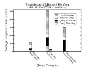
**Figure 7.** Breakdown of miss and hit cost under modified TPC-W with a loaded origin server.
