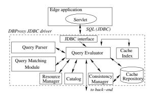
Figure 2. DBProxy key components.
