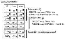
**Figure 4.** Local storage. The local *item* table entries after the queries  $Q_1$  and  $Q_2$  are inserted in the cache. The first three rows are fetched by  $Q_1$  and the middle three are fetched by  $Q_2$ . Since  $Q_2$  did not fetch the  $i\_cost$  column, NULL values are inserted.
