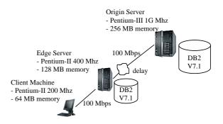
**Figure 5.** Evaluation environment. Three machines were used in the evaluation testbed based on the TPC-W benchmark. The client machine was used to run the workload generator, which applied a load equivalent to 8 emulated browsers. All machines ran Linux RedHat 7.1. Apache-Tomcat 3.2 was used as the app server.
