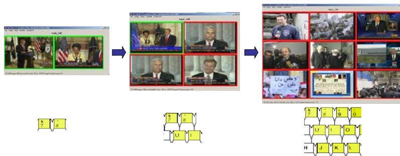
Fig. 2. Manual browsing with different page layouts: 1x2 at the beginning, 2x2 in a later stage, and 3x3 for the rest of the shots. The green bounding boxes indicate the shots labeled relevant, and the keyboard section below a page shows the keys for labeling the respective shots
