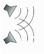
Figure 10: Two speakers out of phase; phases do not add constructively.
