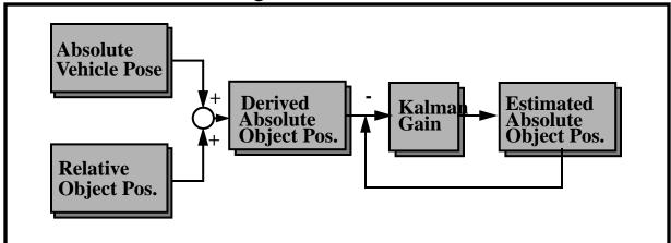
• In position estimation from landmarks, we take the absolute object positions as known and update the position of the vehicle based on it and sensor readings:
