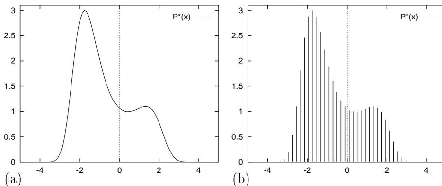
Figure 1. (a) The function  $P^*(x) = \exp [0.4(x - 0.4)^2 - 0.08x^4]$ . How to draw samples from this density? (b) The function  $P^*(x)$  evaluated at a discrete set of uniformly spaced points  $\{x_i\}$ . How to draw samples from this discrete distribution?
