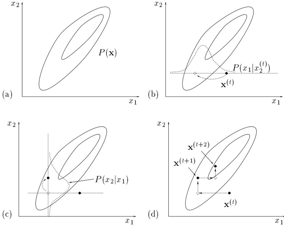
Figure 9. Gibbs sampling. (a) The joint density  $P(\mathbf{x})$  from which samples are required. (b) Starting from a state  $\mathbf{x}^{(t)}$ ,  $x_1$  is sampled from the conditional density  $P(x_1|x_2^{(t)})$ . (c) A sample is then made from the conditional density  $P(x_2|x_1)$ . (d) A couple of iterations of Gibbs sampling.
