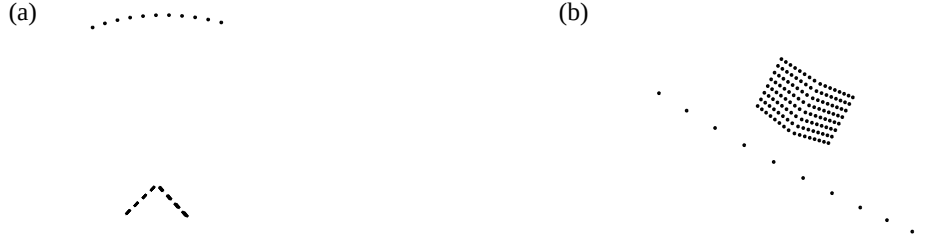
Fig. 8. (a) Plan view of the reference object viewed edge-on (lower) and the arc of successive camera positions in a circle (upper) after transformation to a Euclidean frame. Note the perpendicularity of the planes of the reference object. (b) View from behind the arc of camera positions.
