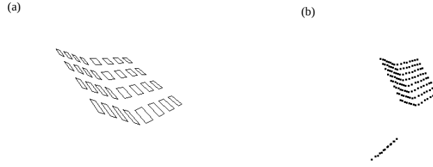
Fig. 7. (a) Structure of the reference object in a coordinate frame with a large projective skew — coplanarity and collinearity are preserved as expected, but the structure is skewed along one plane, and the angle between the two planes is greater than 90^\circ (connectivity has been added to the point structure for illustration). (b) View of the computed structure together with the computed camera positions in the frame with large projective skew. Compare with the plan view after transformation to the Euclidean frame in Figure 8.
