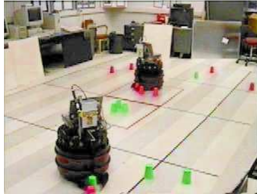
Figure 1: Multi-foraging robots in simulation (left) and in the laboratory (right). In the simulation robots are represented as black circles; arcs indicate the visual sensing range; obstacles are drawn as gray circles; the small discs are attractors. The robots deliver the attractors to the color-coded squares representing delivery areas.
