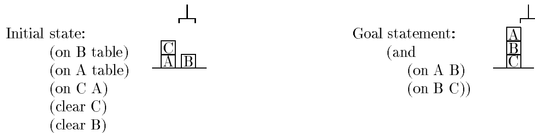
Figure 1 - The Sussman anomaly: Find a plan to transform the initial state to achieve the goal statement.
