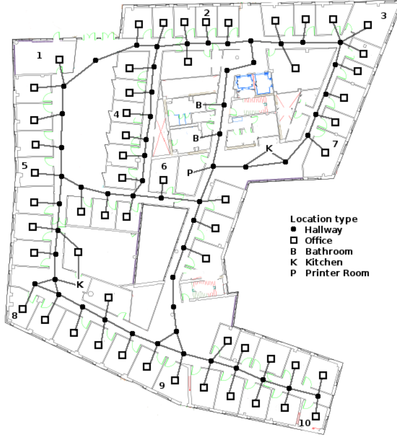
Figure 8.5: Floor plan used in our service robot experiments. The embedded graph represents the map given to the planners. The initial location for the experiments are represented by the numbers 1, \dots, 10 .
