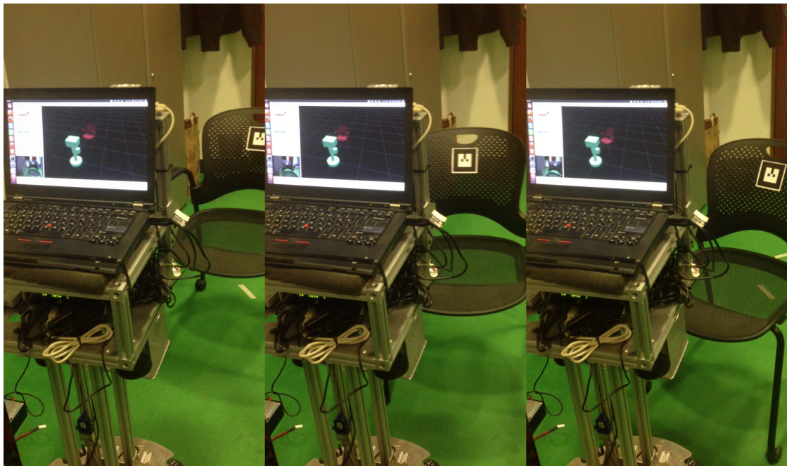
Figure B.1. AR Tag tracking visualization. The simulated chair moves in the world model of the robot as the physical chair moves in the real world.
