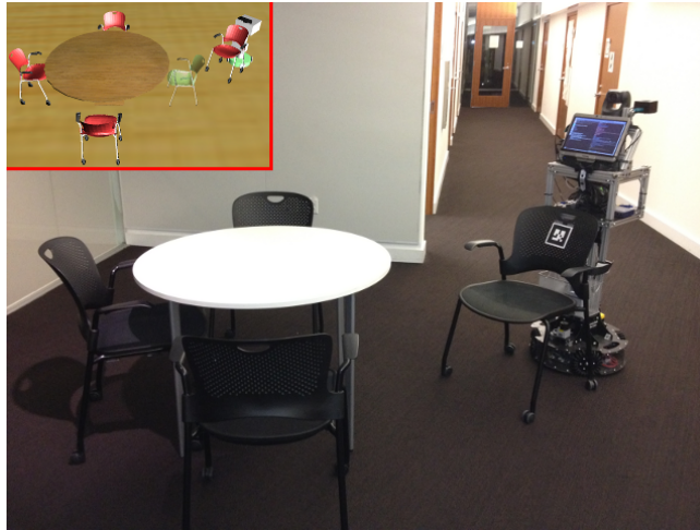
Figure 3.15. A snapshot from one of the real world tests, where the task of the robot is to arrange the chairs around the round table. Visualization of the setup in simulation is provided on the top left corner of the image.
