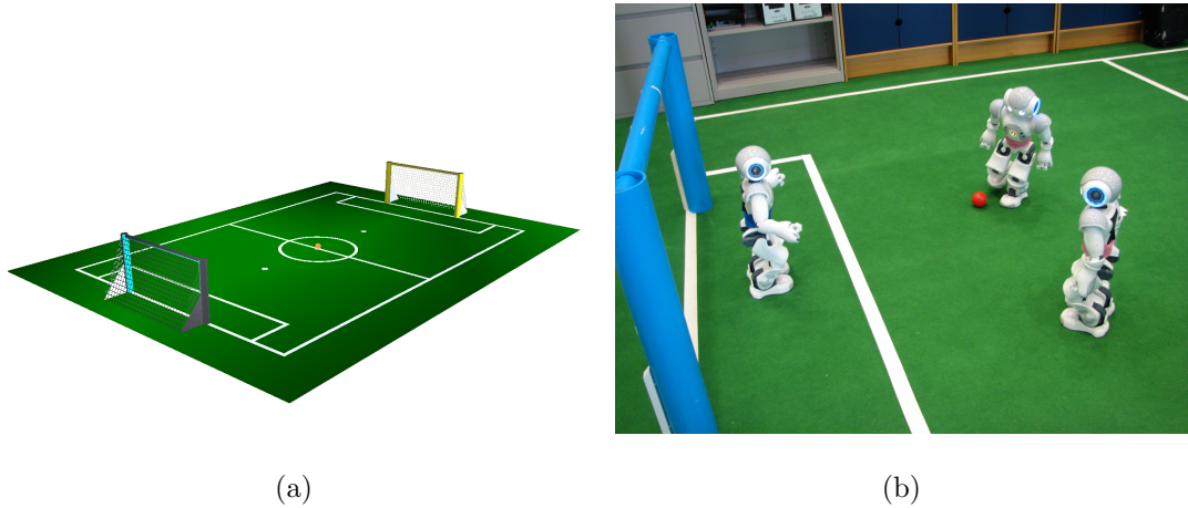
Figure A.1. a) The field setup for the RoboCup Standard Platform League (SPL), and b) a snapshot from an SPL game showing the Nao robots playing soccer.
