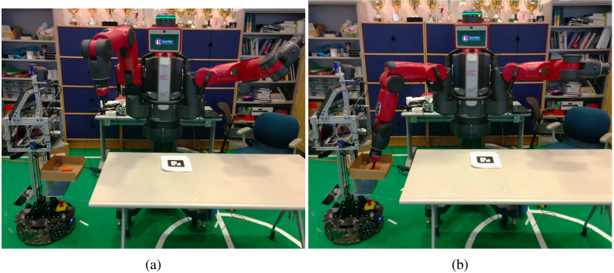
Figure 3.7: (a) CoBot reaches the pick up location while the right arm is waiting and the left arm is waiving. (b) The right arm can now pick up the object.
