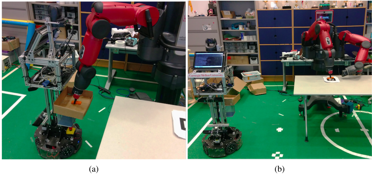
Figure 3.8: (a) Detailed view of Baxter picking up the object. (b) The left arm points at location 1, the right arm drops the object, and CoBot leaves.
