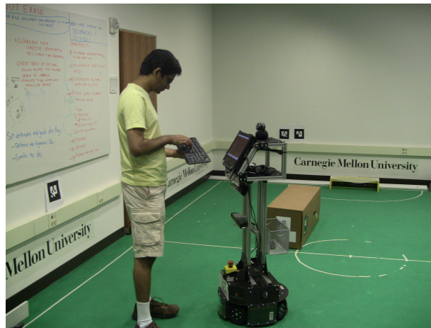
Figure 2.9: A user teaches CoBot to use waypoint navigation to avoid an obstacle.
