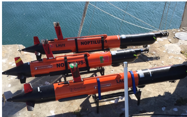
Fig. 1. Three Light Autonomous Underwater Vehicles (LAUVs) from the Laboratório de Sistemas e Tecnologia Subaquática (LSTS) in Porto, Portugal that were used to gather the depth data in Figure 3.
