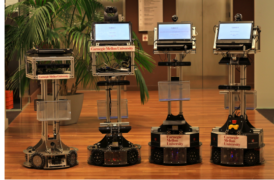
Figure 1: CoBots with omnidirectional motion, onboard computation, interaction interfaces, carrying baskets, and different combinations of depth sensing (cameras and LIDAR).
