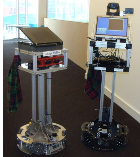
Fig. 1: The CoBot mobile service robots. CoBot robots autonomously perform tasks in human-populated environments, often without any supervision. Autonomous execution monitoring during navigation is thus essential for the safety of people around them.
