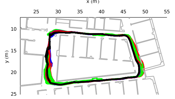
Fig. 5. Combined traces of all successful trials of all approaches: green (KR), red (KS), blue (KC) and black (FSPF). FSPF CGR localization is seen to have the least variation across trials.
