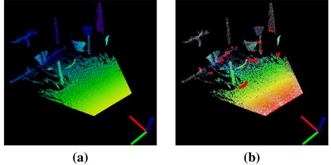
Fig. 2. Obstacle avoidance: The raw 3D point cloud (a) and (b) the sampled points (shown in color), along with the open path limits (red boxes). The robot location is marked by the axes.
