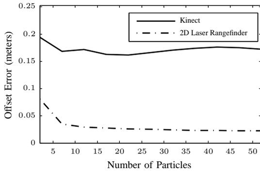
Fig. 3. The offset errors from the true true robot locations while localizing using the Kinect vs. Laser Rangefinder
