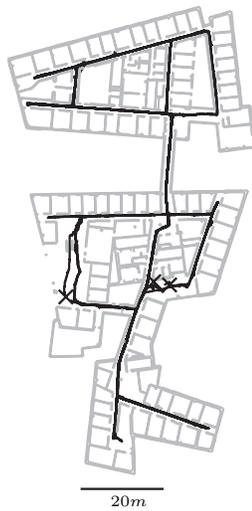
Fig. 4. Trace of robot location for the long run trial. The locations where localization had to be reset are marked with crosses.
