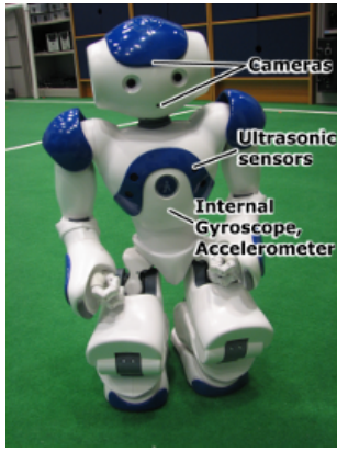
Figure 2: Aldebaran Nao humanoid robot used in the Standard Platform League of RoboCup, and its on-board sensors.
