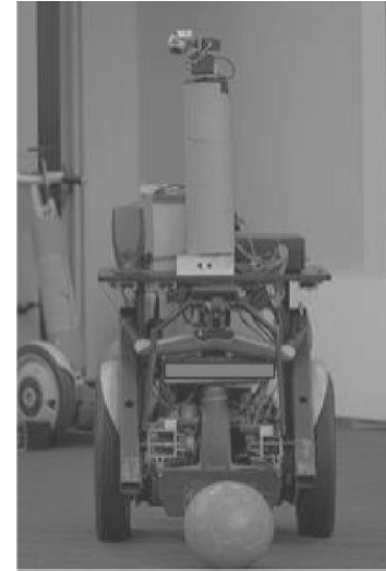
Fig. 3. The Segway RMP soccer robot equipped with a kicker, a catcher, infrared sensors and a camera mounted on a custom pan-tilt unit (Searock et al. 2004).
