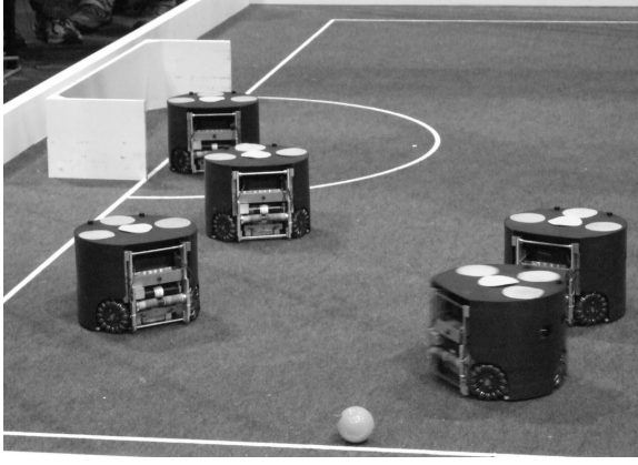
Figure 1: In the Small Size League, two teams with five robots per team compete in a soccer match. The robots use rotating rubber bars to grip a golf ball for “dribbling” and can kick the ball at velocities of up to 10 m/s to pass or shoot on goal. The robots are controlled wirelessly by an off-board computer that tracks all ten robots and the balls using overhead cameras mounted above the field.
