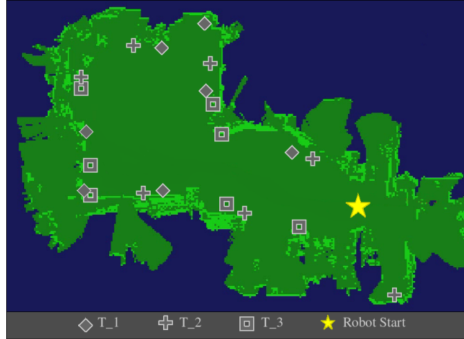
Figure 4: Laser map of Highbay area with different treasure configurations.
