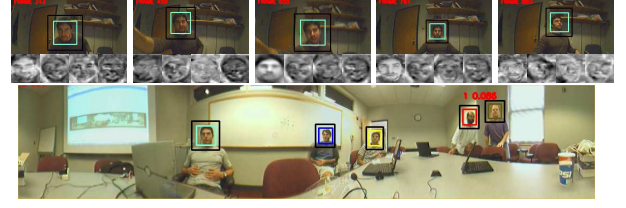
Fig. 5. The inner color box is the output of the face tracker. The black box defines where the face tracker runs.
