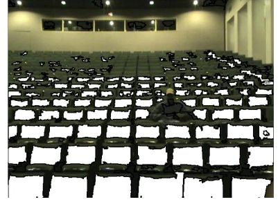
(c) The Generalize function takes the parameters learned from the Grab function and highlights all of the features that match those values (shown in white)
