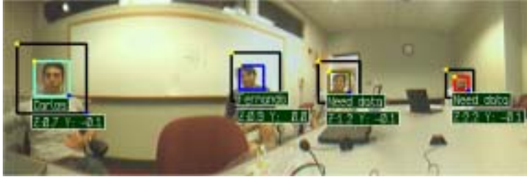
Figure 14: Some images illustrating the depth estimation. In the upper black box the depth( Z ) and the ( Y ) coordinates can be observed.
