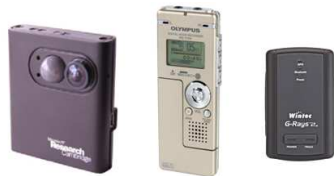
Figure 3. A wearable digital camera, audio recorder, and GPS logger capture the user's experience.
