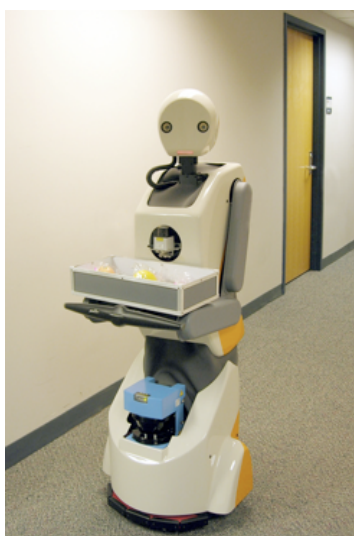
Figure 1. The Snackbot robot, around which the dynamic snack delivery service is based.
