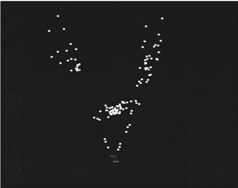
FIG. 7. Showing an overhead view of the recovered structure using the image pair shown in Figs. 6a, 6b. The camera centers are located at the apex of the parabola. It can be seen that the points all lie close to a quadric surface, indicating that they may lie on a critical surface.
