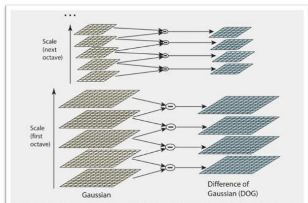
Figure 1: For each octave of scale space, the initial image is repeatedly convolved with Gaussians to produce the set of scale space images shown on the left. Adjacent Gaussian images are subtracted to produce the difference-of-Gaussian images on the right. After each octave, the Gaussian image is down-sampled by a factor of 2, and the process repeated.
