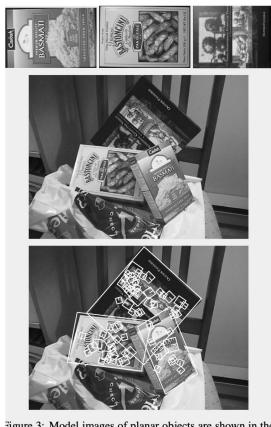
Figure 3: Model images of planar objects are shown in the op row. Recognition results below show model outlines and mage keys used for matching.
