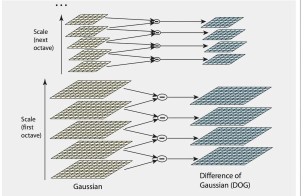
Figure 1: For each octave of scale space, the initial image is repeatedly convolved with Gaussians to produce the set of scale space images shown on the left. Adjacent Gaussian images are subtracted to produce the difference-of-Gaussian images on the right. After each octave, the Gaussian image is down-sampled by a factor of 2, and the process repeated.
