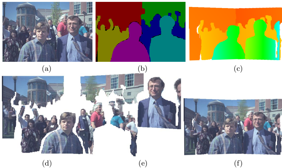
Fig. 9. Results on the symposium sequence: (a) third of five images; (b) initial segmentation into six layers; (c) recovered depth map; (d) and (e) the five layer sprites; (f) re-synthesized third image (note extended field of view).
