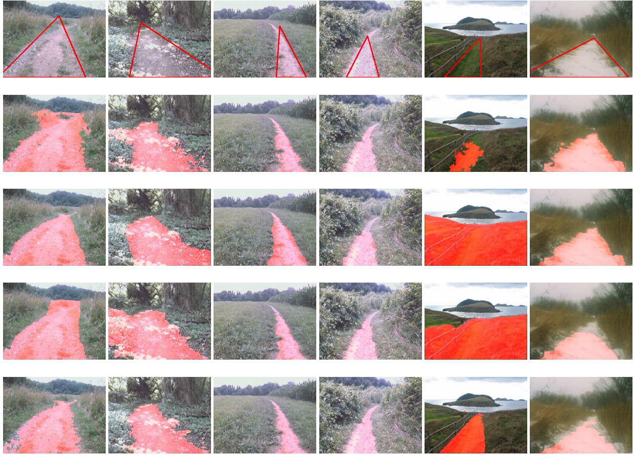
Figure 2. Trail refinement results of the methods. Rows show initial models, refinement results of the of the superpixel method, GrabCut, regular graph cut, and graph cut with distance penalty method, respectively. Left 4 columns include images from Set-1 and, right 2 columns contain images from Set-2.
