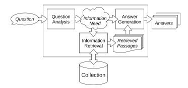
Figure 1.1: A QA system, consisting of an IR system encapsulated by NLP components: front-end Question Analysis and back-end Answer Generation.
