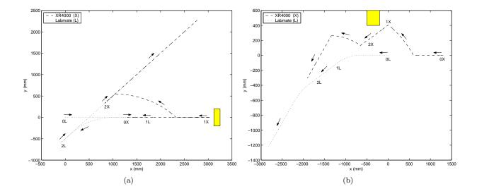
Figure 6: Experiments: (a) the XR4000 resigns the leadership (1X) and receives it back (2X); (b) the XR4000 requests the leadership (1X) and returns it (2X) to the Labmate.
