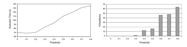
Figure 8: Completion time and number of deadlocks varying the threshold  $\tau$ .
