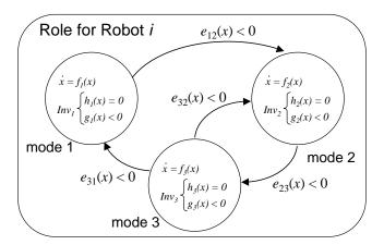
Figure 2: Schematic of a role composed by three roles (modes). Each mode is characterized by differential equations and algebraic constraints. The conditions under which transitions between modes occur and the conditions under which the robot stays in a particular mode are specified by the guards and invariants respectively.
