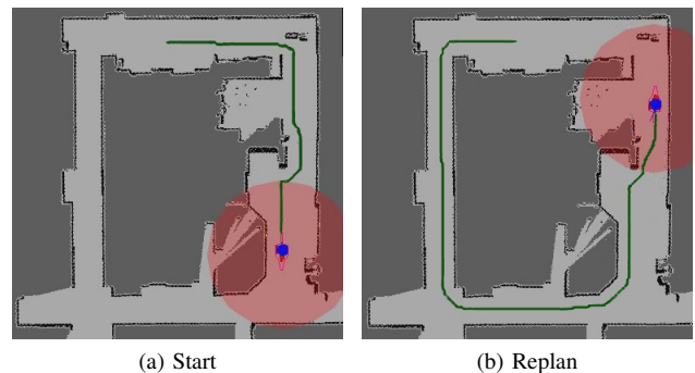
Fig. 9: (a) the robot initially plans a path through the upper right corner to the goal. (b) once the robot reaches the corner it discovers that it cannot maneuver past the obstacles and plans a path around the loop, leaving a 3-D circle at its present location.
