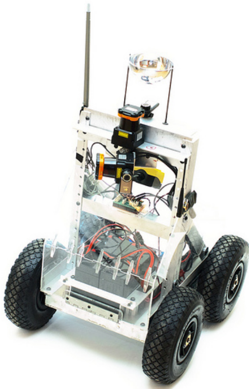
Figure 8. One of the University of Pennsylvania's MAGIC2010 robots. The robots used two laser range scanners, an omni-directional camera, and a panning camera to gather information about the environment. An on-board Mac Mini provided computational power, and a 802.11 antenna provided the data link with the ground control station (GCS). (Photo ©2010 Paul Vernaza)
