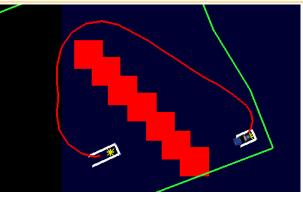
2D (x,y) distance accounting for obstacles (single Dijkstra's on 2D grid cell starting at goalcell will give us these values)
