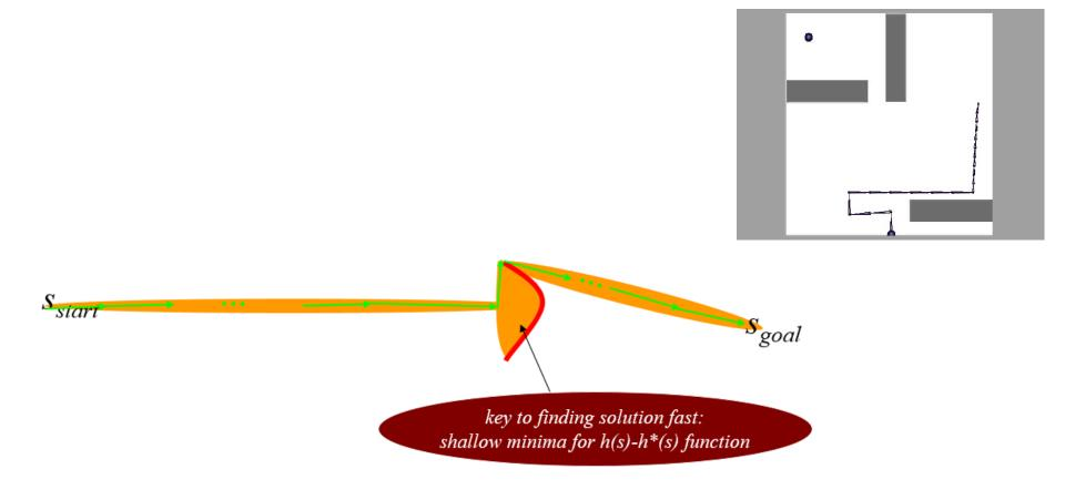
• 20DoF Planar arm planning (forget optimal A\*, use weighted A\*):
