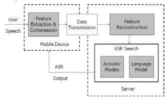
Figure 3: System architecture when the speech recognition is split across the mobile device and the server. Feature extraction is done on the mobile device, and the ASR search is implemented on the server [12]
