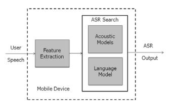
Figure 1: System architecture when both the feature extraction and the ASR search are implemented on the mobile device alone [12]
