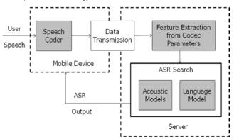
Figure 2: System architecture when both the feature extraction and the ASR search are implemented on the server end with mobile devices encoding the speech signal before transmitting the encoded bits to the server [12]
