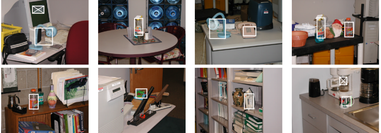
Figure 2: Sample test images for the indoor detection task. White empty squares indicate correct detections by our system described in § 5.3, while squares with a cross indicate false positives.
